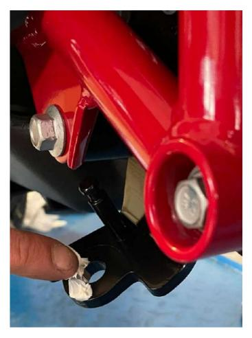
Lubricate the screw with grease and tighten to a tightening torque of 20 Nm
