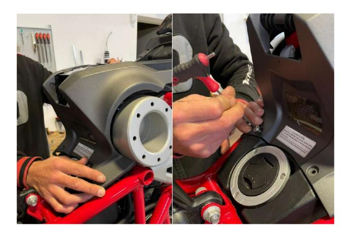
Reposition the saddle and fix the 4 screws.
