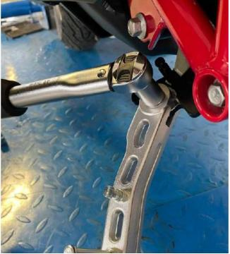
Position the safety switch as indicated and tighten the M6 screw with a torque of 10 Nm
